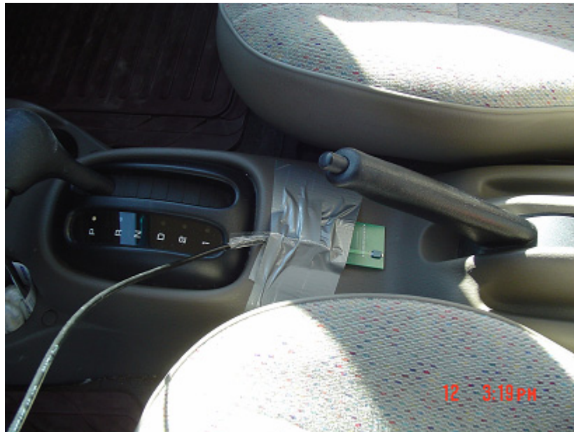
Figure 17: Receiving antenna on the gearbox
