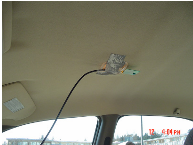
Figure 19: Receiving antenna under the dome light
