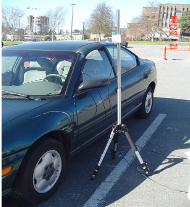
Figure 13: Antenna positioner (at roof height)
