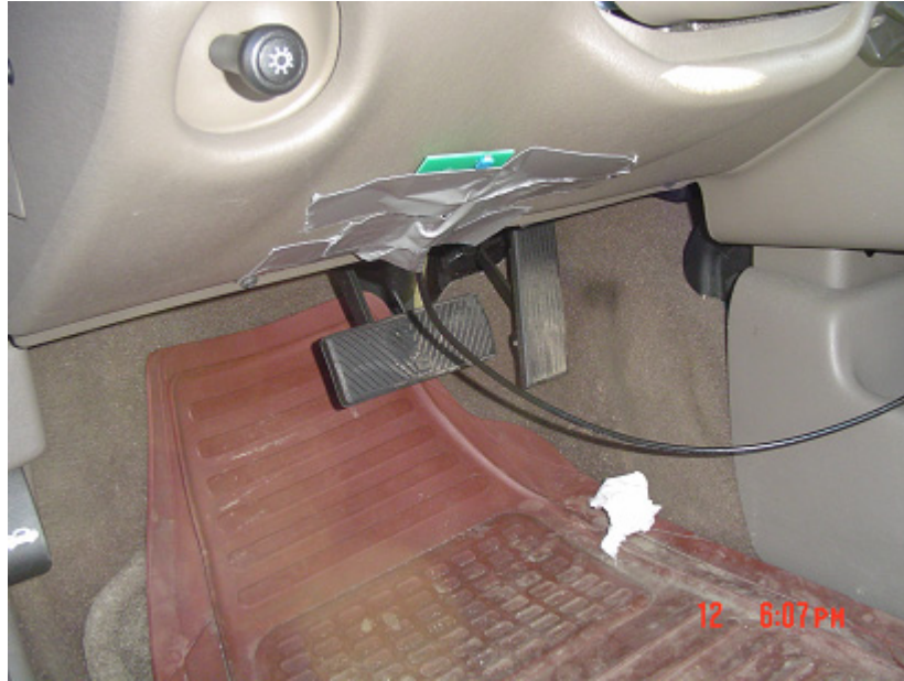
Figure 18: Receiving antenna under the steering wheel
